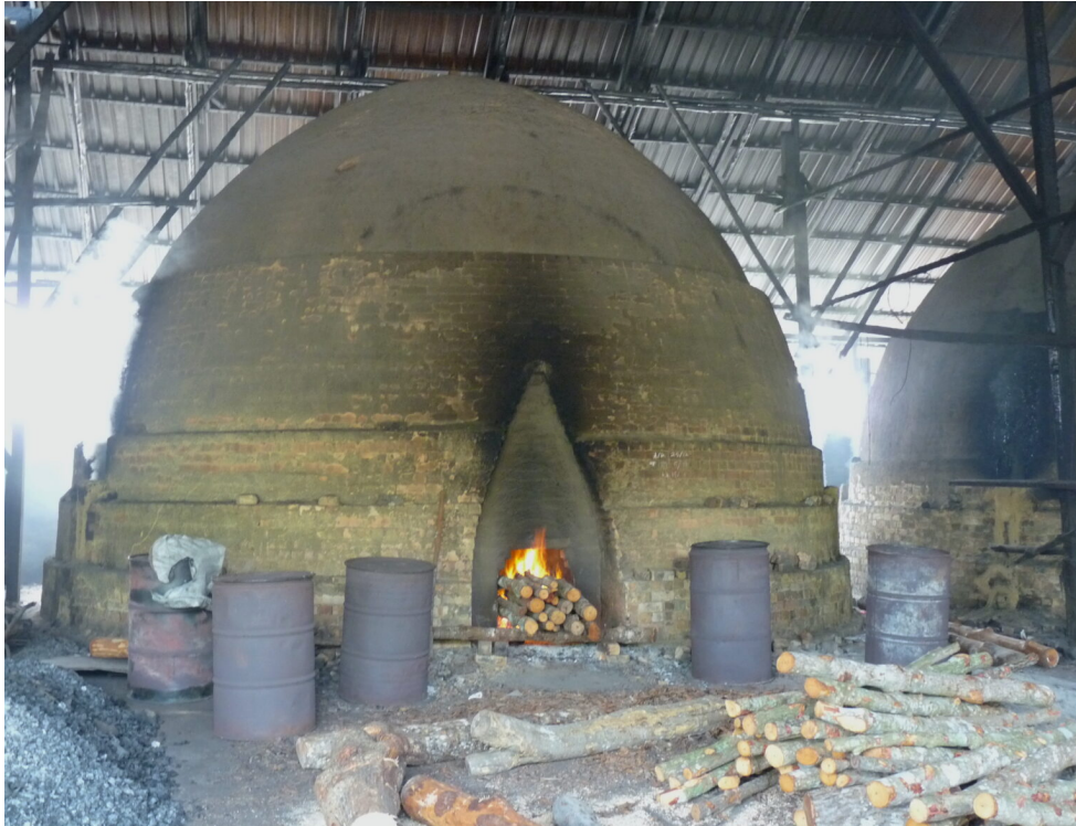
A charcoal kiln in Malaysia. Image courtesy of Behara Satyanarayana
